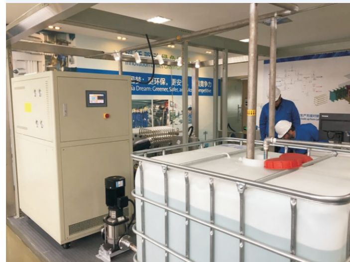
Dynamic temperature control system apply to Corning Advanced-Flow™ glass reactor
