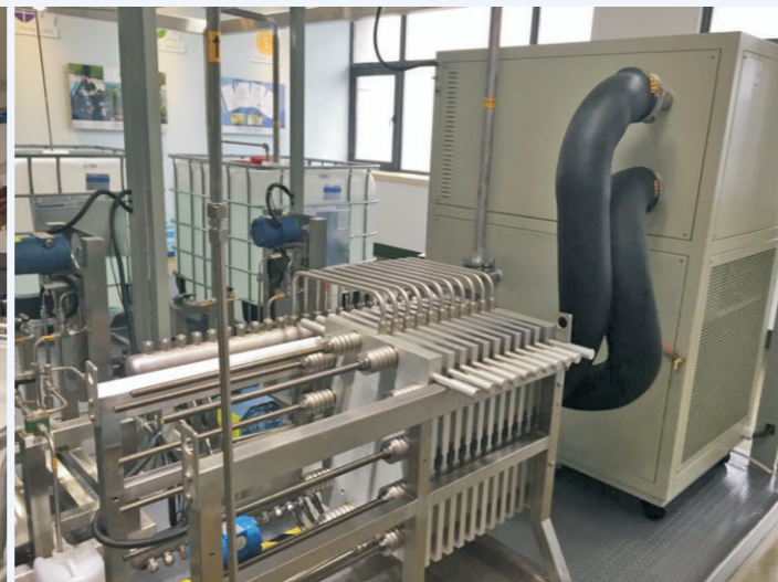
Dynamic temperature control system apply to Corning Advanced-Flow™ glass reactor
