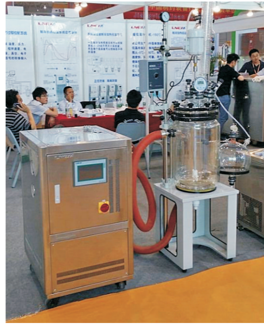
Dynamic temperature control system apply to Corning Advanced-Flow™ glass reactor
